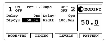
If you need to specify a unit for a parameter, simply press the appropriate unit key (NANO, MICRO/MEGA, MILLI/KILO) instead of the ENTER key.
