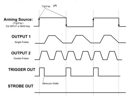
NOTE The PLL cannot be selected as the arming source. Select continuous pulses mode with the PLL as PERIOD SOURCE to achieve the same result.
