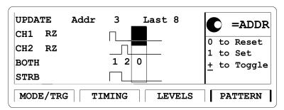
While the entry focus is in the bit-edit window you can use the knob to scroll through the data.
