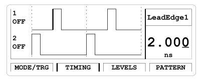
Set the transition time for the leading edge of the pulse, measured from 10% to 90% of the pulse amplitude.
