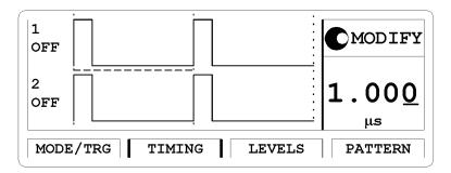
Note that in graphics mode you can only adjust the values of each parameter, not the parameter format. If you want to change the format of a parameter, for example Width to DutyCycle, you must be in text mode to select the parameter name with the cursor.
