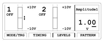
Use the Levels screen to view and control the pulse-level parameter for both channels on one screen. If you have a single channel instrument both the timing and level parameters are displayed on the Output screen (see "The Output Screens" on page 106).
