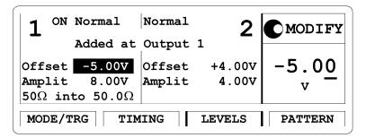
The Levels graphic page is also modified to indicate the multiple levels formed by outputs 1 and 2:
