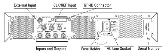
With option UN2 the major inputs and outputs of the instrument (as described in "*The Front Panel*" on page 18) are available at the rear panel:
