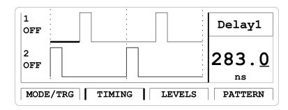
Set the delay of the leading edge within the pulse period. There are three delay formats available:
