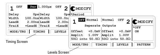
Press the TIMING OR LEVELS softkey to access these screens. In the Timing screen you can set up the clock frequency and, for output 1 and 2, the timing for the signals (delay, pulse width, duty cycle, ...).
