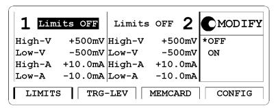
After you switch on the limits, the pulse level parameters on the Levels/ Output screens cannot be adjusted outside the ranges specified on the Limits screen if the output is switched on. Note that because current and voltage limits apply, the available ranges of the impedance parameters are also affected.
